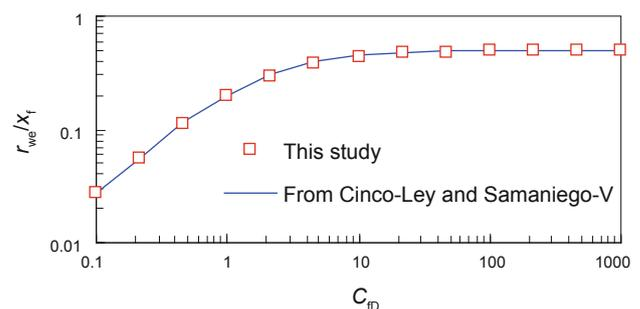
Fig. 2 A comparison of equivalent wellbore radii from different models
