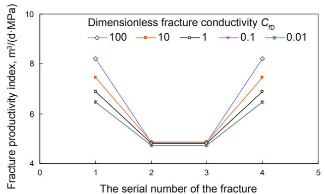
**Fig. 4** Curves of productivity index varying with  $C_{fd}$
