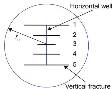
**Fig. 3** Schematic of the fractured horizontal well (after Raghavan and Joshi, 1993)
