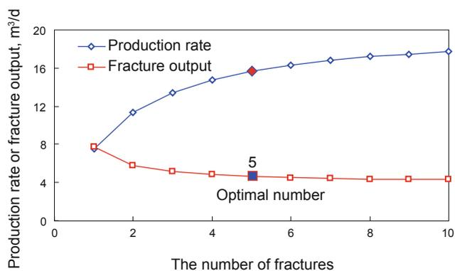
**Fig. 6** Production rate and fracture output varying with fracture number
