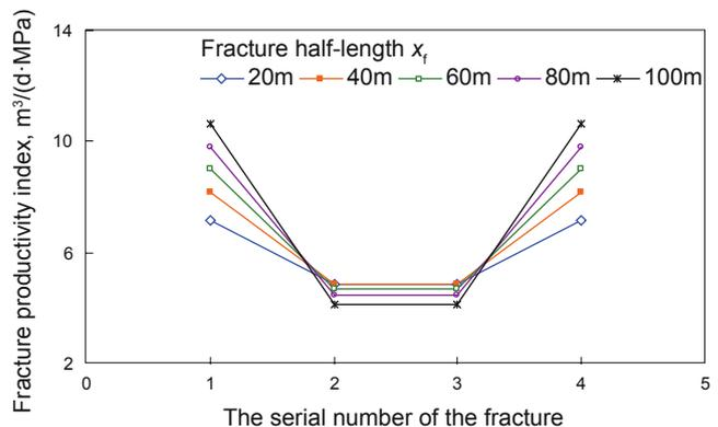
**Fig. 5** Curves of productivity index varying with  $x_f$  values
