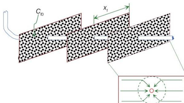
Fig. 1 Schematic of flow regimes in the fracture
