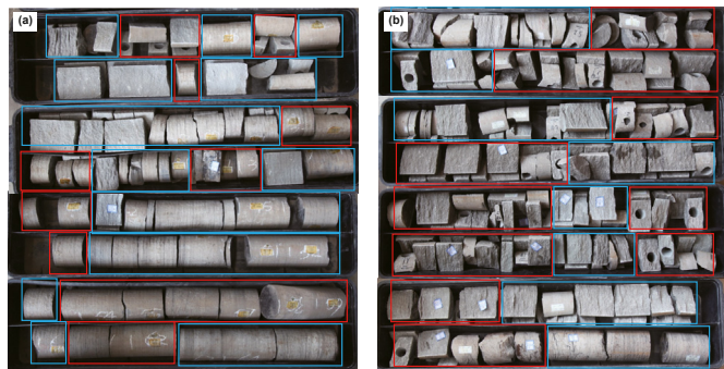
Fig. 2. Interbedded oil-bearing (red lines) and oil-free (blue lines) sandstones in the Chang 7 Member. (a) Well A, 2138–2144.04 m core; (b) Well B, 2193.92–2208.22 m core.
